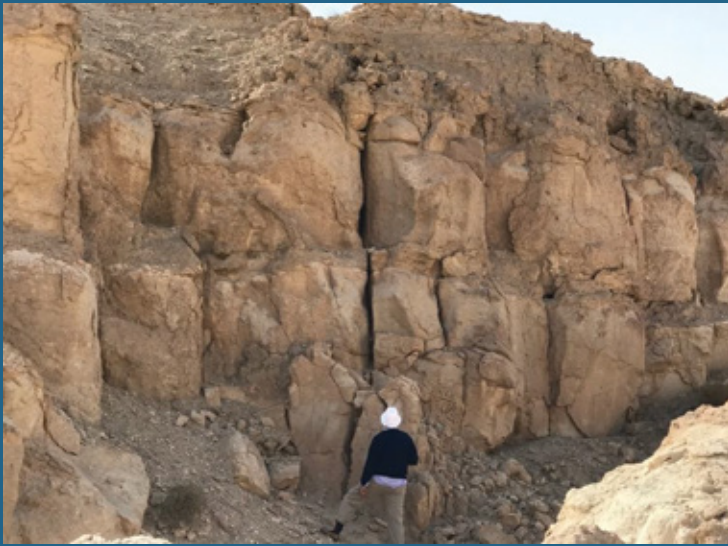
Figure 5. One single joint cutting through both stiff and softer units. Notice the majority of the joints are constrained only within the stiff (light color) unit.
