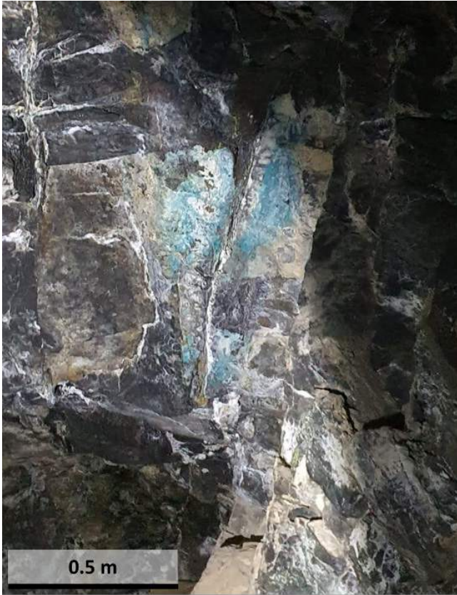
Image 7. Remaining copper oxide at surface of mined-out fracture plane.
