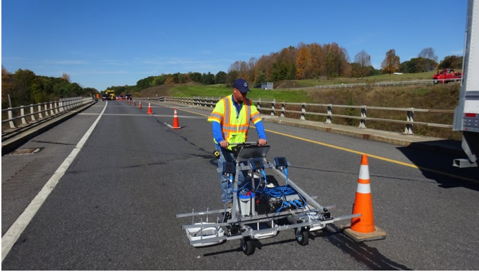
GPR method is used to identify bridge and road damages (photo from Infrastructure Preservation Corporation website)
