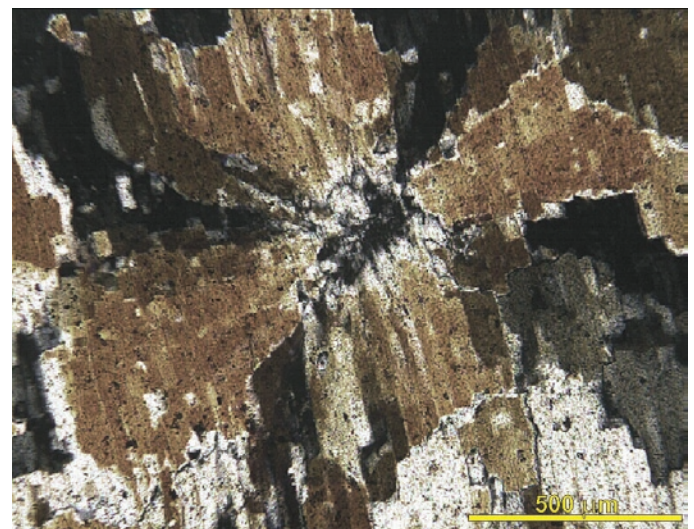
Polarized light microscopy; hyperblastic textures of quartz crystals (#O2; longitudinal radial cut).
