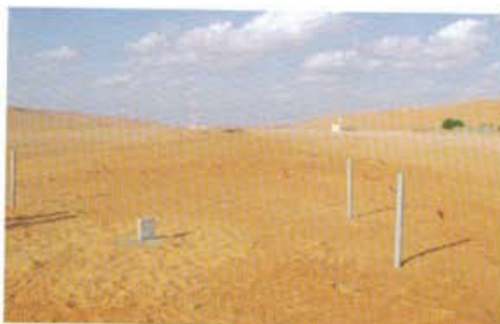
Figure 5 PDO sand trap near Al Raha camp situated on a small dune in the interdune area between two linear dunes Sharqiyah Sands.
