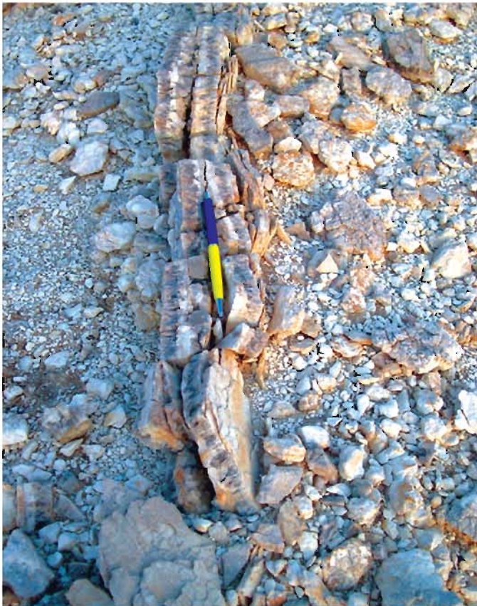
Calcite filled veins crosscutting the main regional seal of the Fiqa Formation
